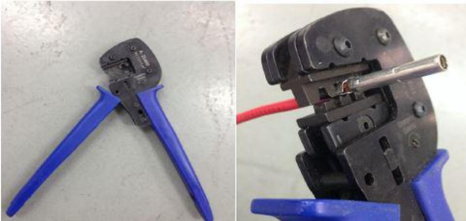
◆ Insert the assembled cable into male/female connector. A "chick" sound can be heard when connecting correctly. Then tighten the cap. Refer to the picture below.
