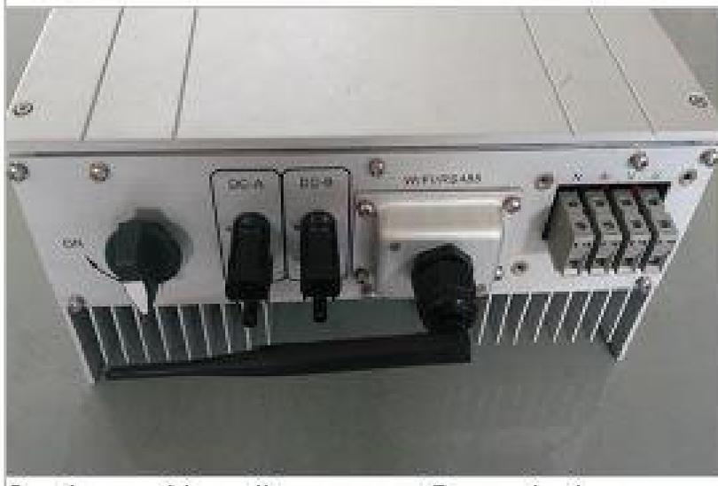
2. Disconnect the DC and AC breaker, DC switch in the "OFF" state.
