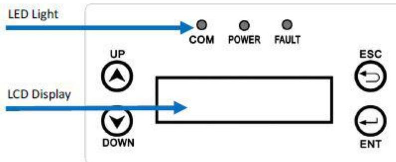
There are four function keys on the front panel: UP, DOWN, ESC, ENT. The keypad is used for:
